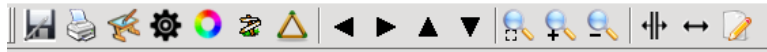
Figure 7.23: The toolbar for the Spectral Profile tool allows the user to save the spectrum, print or save the tool as an image, edit preferences (general, tool, legend), spectral smoothing, pan or zoom around the spectrum, select a range of interest, jump to a channel, or add a label.
